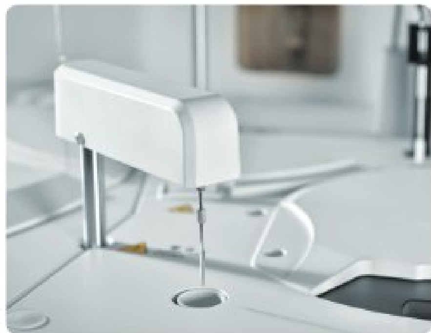
Independent mixing bar
