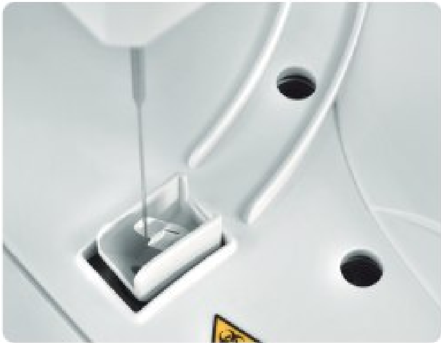
Waterfall probe cleaning
